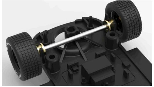
Actually the chassis design is not to blame. The guide is a snap in unit that pops up through the hole shown here in front of the axle. The axles are very strong and the wheel bushings seat nicely in the chassis mount. This is a well-made slot car. The guide pin however is sloppy as all hell. It binds from time to time because the pickup wires can get caught on the guide pin post.
