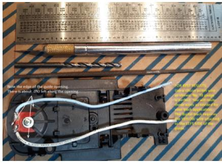
This is the finished chassis. The area marked here will give you an idea just how much you will remove from the guide hole.
