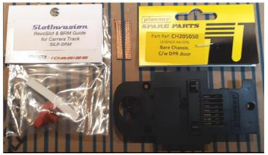
The bare chassis, or your car's chassis. You are going to make adjustments to the guide pin area only, so I suggest you remove the front axle for this part of the modification. You need the SlotInvasion BRM/Revo kit as shown. You will also need a set of brushes. I cut these from Pioneer UltraBraid [R]. The length should be 1 1/4 inches to start. You will trim these later. Look at your chassis carefully; the guide pin area resembles the letter "C". It is this
